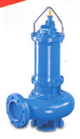
"AMU" Low Speed Heavy Duty Sewage and Effluent Submersible Pump is Vertical single casing pump with non clog, channel type impeller for handling of unscreened large solids. Squirrel cage induction motors specially manufactured by "AMU" with Class 'F' and Class 'H' insulation suitable upto 155°C and 180°C for 20 Starts and Stops per hour. "AS" Pumps are also available with cooling Jacket arrangement for Dry Pit as well as Wet Pit installation with auto coupling arrangement.
