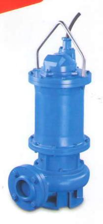
"AMU" High Speed Light Duty Sewage and Effluent Submersible Pump is Vertical single casing pump with non clog, channel type impeller for handling of screened sewage. Squirrel cage induction motors specially manufactured by "AMU" with Class 'F' and Class 'H' insulation suitable upto 155°C and 180° C for 15 starts and stops per hour. "ALS" Pumps are also available with auto coupling arrangement.
