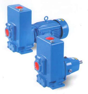
"AMU" Centrifugal Self Priming Pumps are non clog, bare shaft, heavy in weight for sturdiness and better long life. 'AEP' Pumps are back pull out type construction & fitted with sufficient size of 'passage to pass solids from the casing. These are most popular and suitable for any kind of dirty water application. These pumps are fitted with Mechanical Seal to ensure zero leakage.
