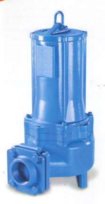
"AMU" Heavy Duty Sewage and Effluent Submersible Pump is Vertical single casing pump with vortex type impeller for handling of unscreened large sewage. Squirrel cage induction motors specially manufactured by "AMU" with Class 'F' and Class 'H' insulation suitable upto 155°C and 180°C for 15 Starts and Stops per hour.
