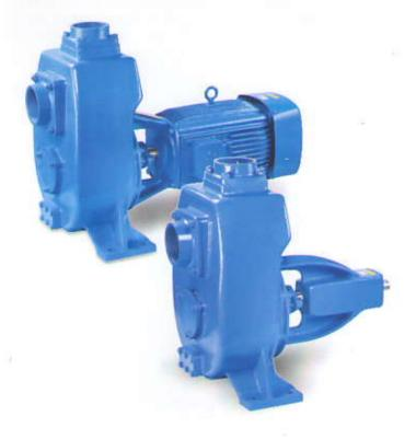
"AMU" Centrifugal Self Priming Pumps are non clog, bare shaft, heavy in weight for sturdiness & better long life. 'ASP' Pumps are back pull out type construction & fitted with sufficient size of passage to pass solids from the casing. These are most popular & suitable for any kind of dirty water application.
