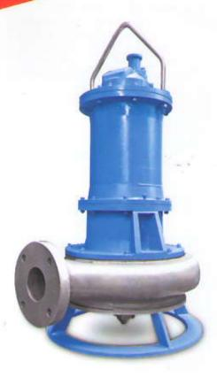
"AMU" Low Speed Heavy Duty Submersible Pump is Vertical single casing pump suitable for all kind of slurries. 'ASR' Pumps are designed for continuous operation in tough abrasive heavy industry applications. The pump features high chrome iron construction for liquid end components such as the casing, agitator, wear plates & impeller which are designed for long service life in tough applications where other pumps of inferior construction may fails.
