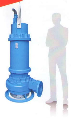
"AMU" Low Speed Heavy Duty Submersible Pump is Vertical single casing pump closed type impeller for handling of raw / turbid water. Squirrel cage induction motors specially manufactured by "AMU" with Class 'F' & Class 'H" insulation suitable upto 155°C & 180°C for 20 Starts & Stops per hour. 'ACS' Pumps are also available with auto coupling arrangement for vertical installation.
