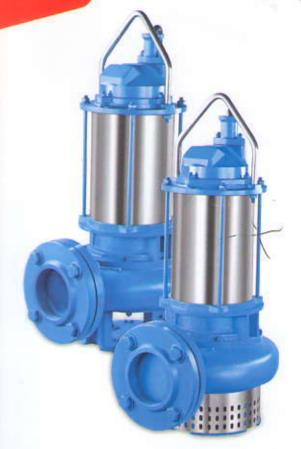
"AMU" Low Speed Heavy Duty Sewage and Effluent Submersible Pump is vertical single casing pump with non clog, channel type impeller for handling of unscreened sewage. Squirrel cage induction motors specially manufactured by "AMU" with Class 'F' and Class 'H' insulation suitable upto 155°C and 180°C for 20 Starts and Stops per hour. 'ASE' Pumps are also available with auto coupling arrangement.
